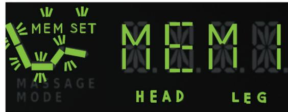
**NOTE:** When the new position of the head is higher than the current position of the head, first the head section and then the leg section move to the corresponding memory position.
